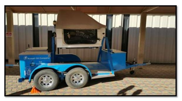
Compact pickup truck cab affixed to a two-axle low profile trailer. Acceleration and braking control systems spin the cab to simulate a rollover accident. The Rollover Simulator is an aide in teaching people the necessity of using seatbelts to avoid serious injury in a car crash resulting in a rollover. The "dummies" in the simulator that are not restrained by a seatbelt are thrown from the simulator in a terrifying real enactment of the deadly results of seatbelt negligence.
